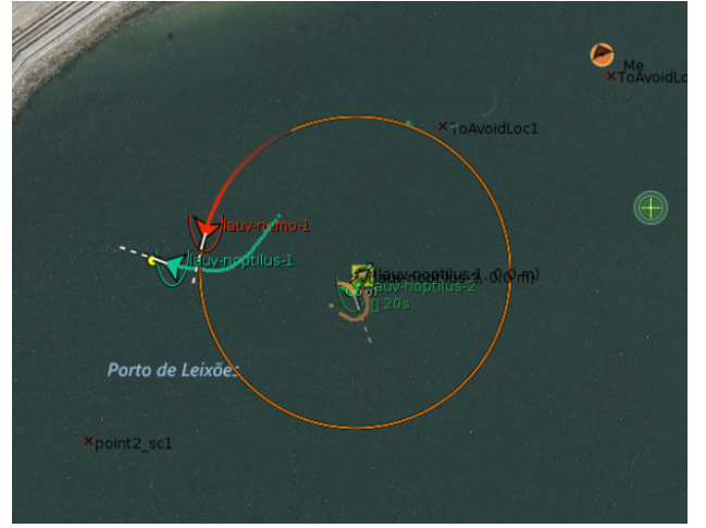
Fig. 2. Neptus console. Simulated target follows a loitering maneuver while the LAUV executes the Robust MPF controllers.
