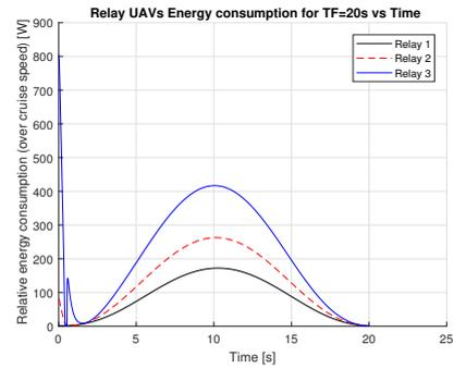
Fig. 10. Estimated relative energy consumption for arrival time=20s.
