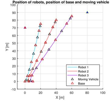
Fig. 5. Motion simulation for 3 Relay-UAVs platoon deployment
