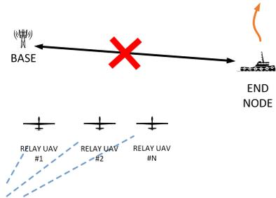
Fig. 2. First stage. Communication between the base and moving vehicle is denied and an additional set of UAVs are ready to act as relay nodes
