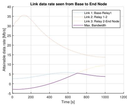
Fig. 8. Estimated link data-rate for 2 Relay-UAV's platoon deployment motion simulation. Non-dashed line is the effective attainable bandwidth
