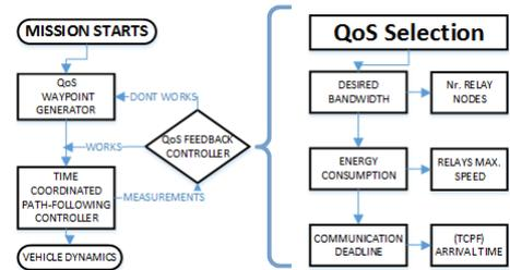
Fig. 1. Algorithm (left) and QoS selection (right) workflow.
