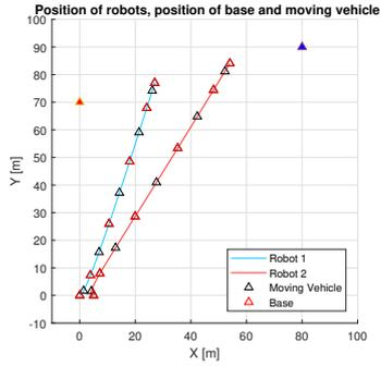
Fig. 7. Motion simulation for 2 Relay-UAV's platoon deployment
