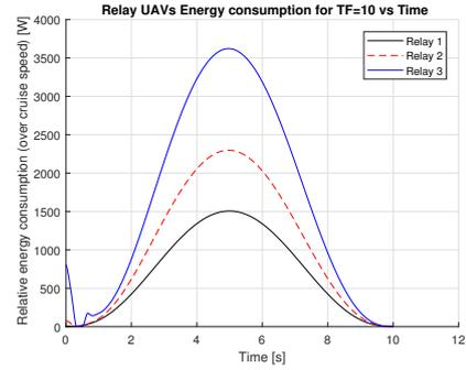
Fig. 9. Estimated relative energy consumption for arrival time=10s.
