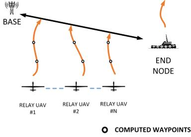
Fig. 3. Second stage. Communication between the base and moving vehicle is enabled thanks to the additional set of UAVs following the path composed by the computed waypoints.
